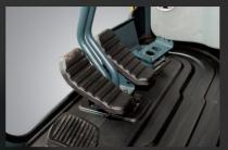
The foot rest, attachment pedal, left and right travel pedals and boom swing pedal are configured for convenient access.
