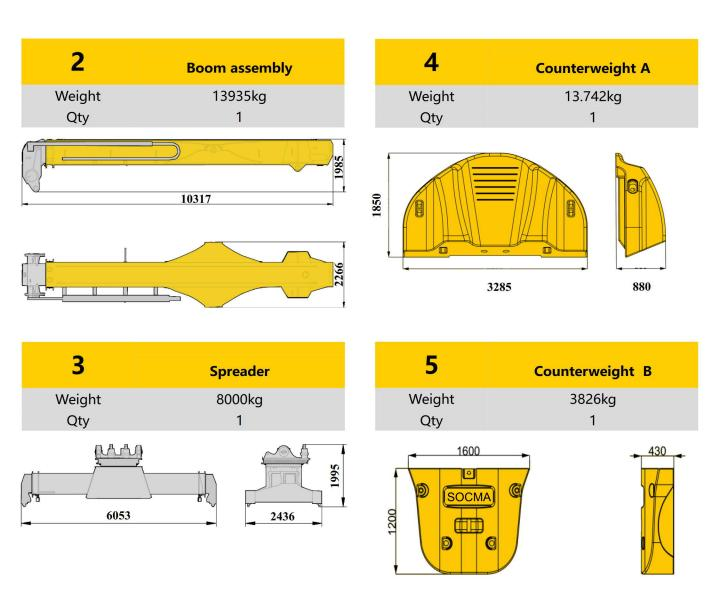
NOTES: All of these are single piece weight, and boom assembly include boom and telescopic cylinder.
